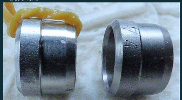
Pic 3: Cutting rings in Duplex (1.4462) hardend with/without SuperExpanite
