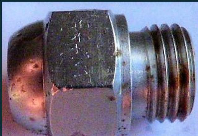
Pic 5: SuperExpanite treated nozzle out of 303 (1.4305)
