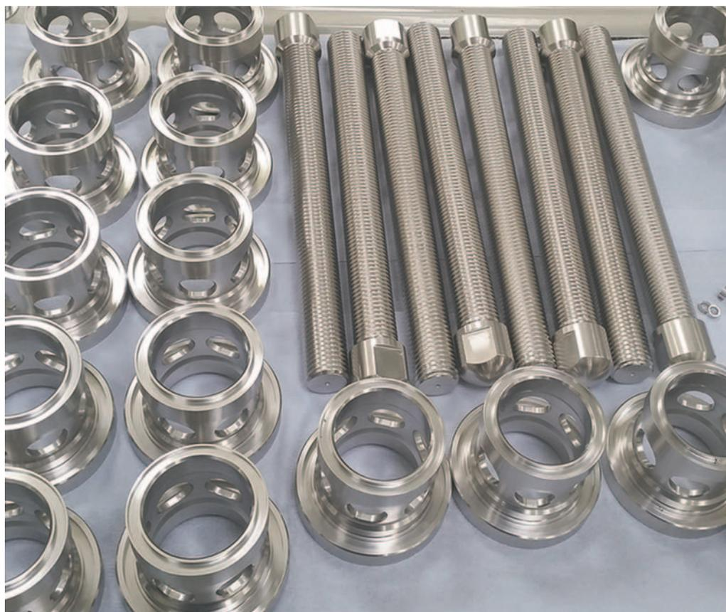
"In cooperation with Expanite we relatively quickly found a hardening that made our surface resistant against scratches and corrosion. The solution passed our test in service where the system remained sealed and tight and in addition the solution was also easy and cost efficient to implement."
