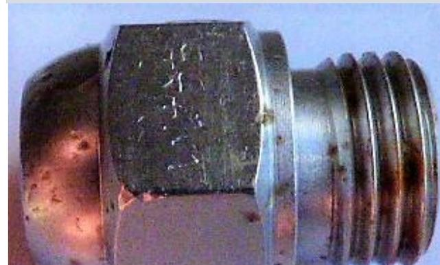
Pic 5: SuperExpanite treated nozzle out of 303 (1.4305) component
