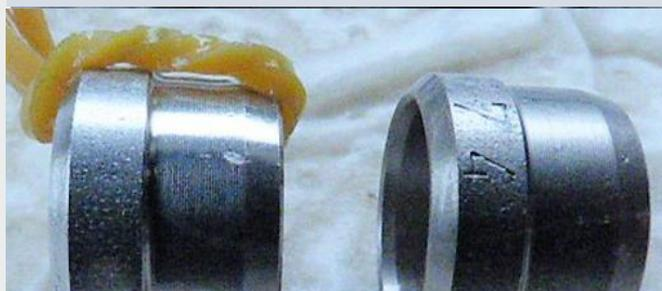
Pic 3: Cutting rings in Duplex (1.4462) hardend with/without SuperExpanite
